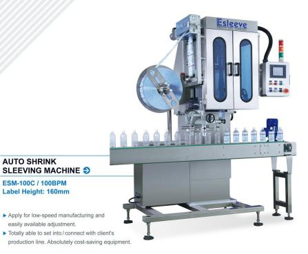
L1204mm × W910mm × H1832mm (able to reach the height to 2398mm) Machine Dimension 2.5KW Approx. Power Consumption
